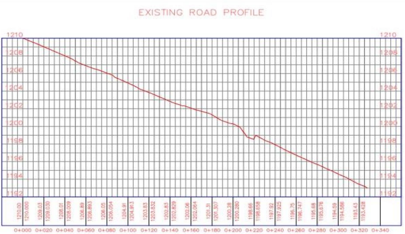
Figure 13: Existing road profiles
