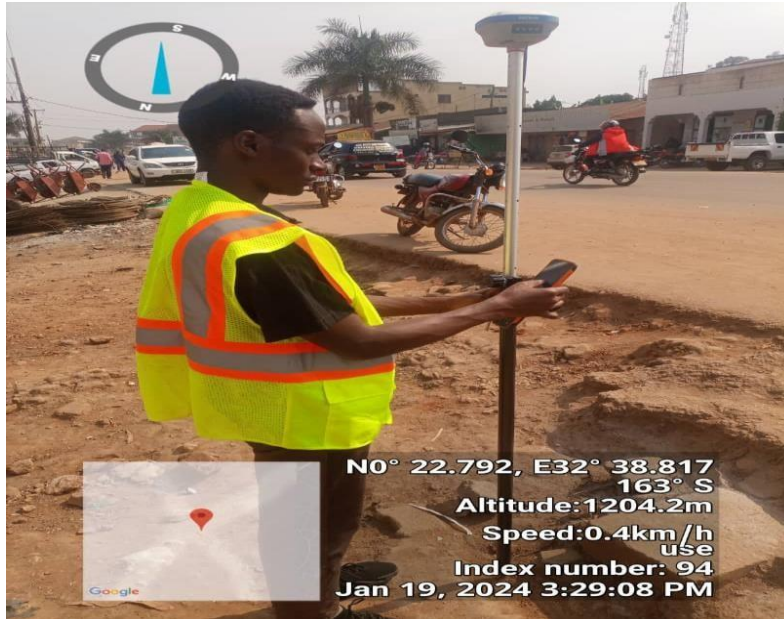
Figure 8: Getting Elevations during Topographic surveys
