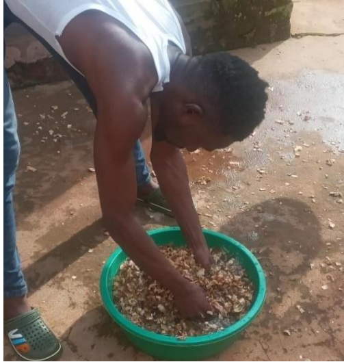
Washing the raw Sawdust
