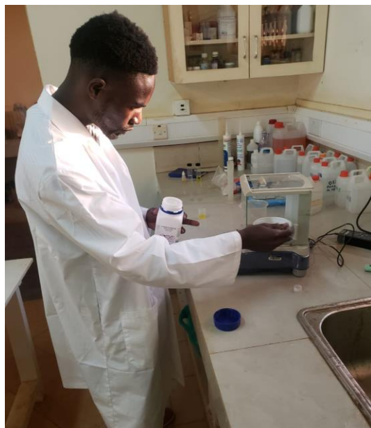
Weighing NaOH for base preparation
