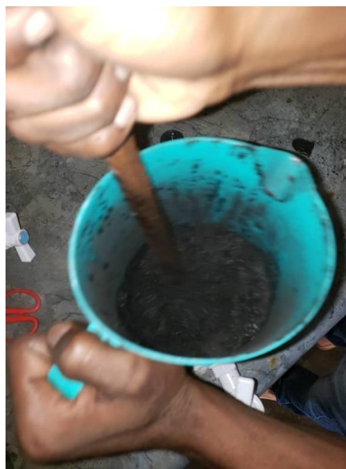
Impregnating the carbon with acid
