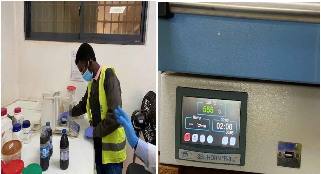
Figure 13: Taking weight of sludge samples using a weighing scale and a muffle furnace ignited sample at 555°C for 2hrs for TVS determination.
