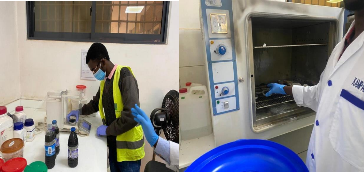
Figure 26: Weighing the faecal sludge samples Figure 27: Placing sludge samples in an Oven
