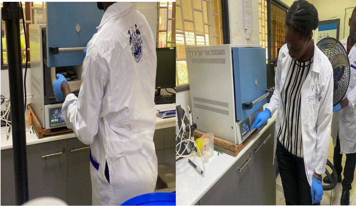
Figure 24: Placing samples in muffle furnace. Figure 25: Setting the muffle furnace at 550°C
