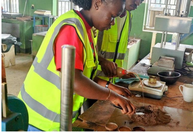
Figure 6:sample preparation for the Atterberg limit test
