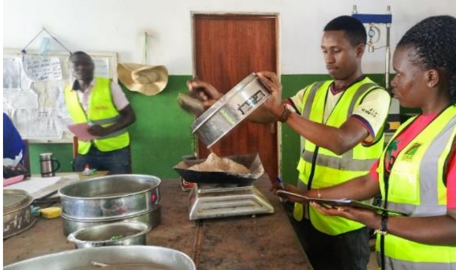
Figure 8: grain size analysis test for the river sand
