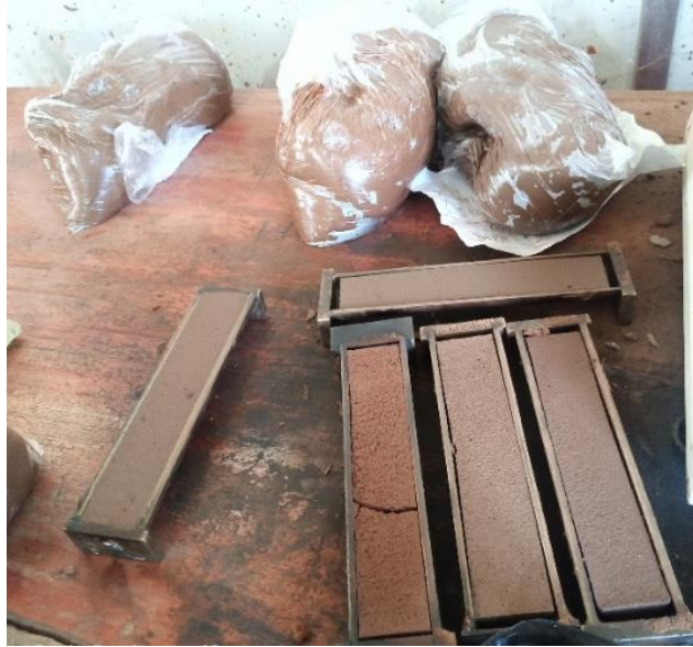
Figure 7: linear shrinkage molds containing soil sample
