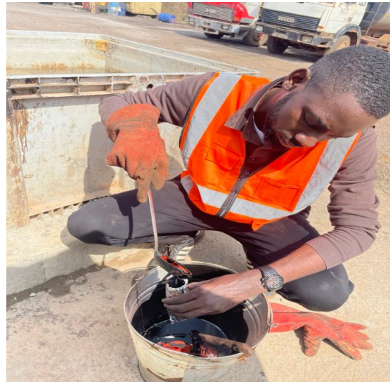
appendix 13 Storage stability test
