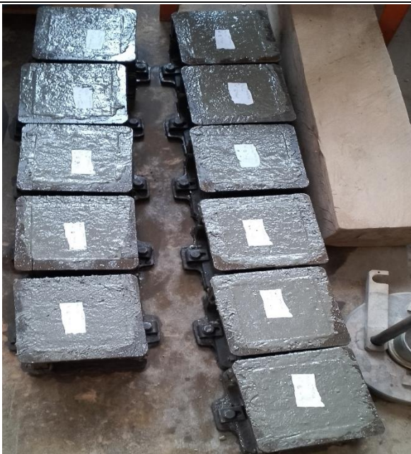
Appendix Figure K-7: Freshly cast concrete left to harden
