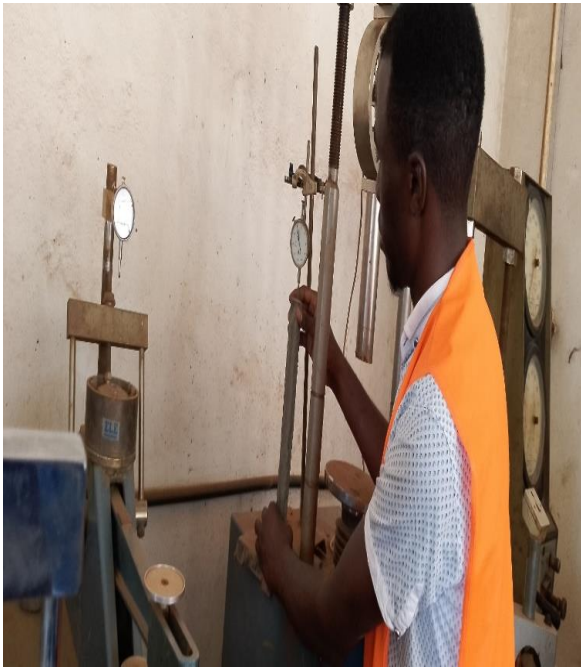
Appendix Figure K-5: Measurement of length changes of the concrete bars, using a dial Gauge
