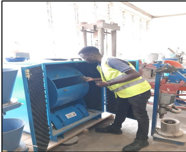
Figure 3-4 Operation of the Steel drum to carry out LAAV test
