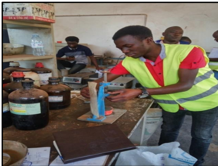
Figure 3-2 Operation of the Vicat Apparatus for setting time test
