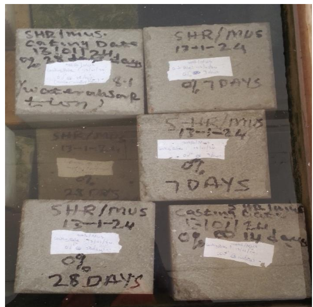
Appendix Figure K-8: Hardened concrete in soaking tank for curing
