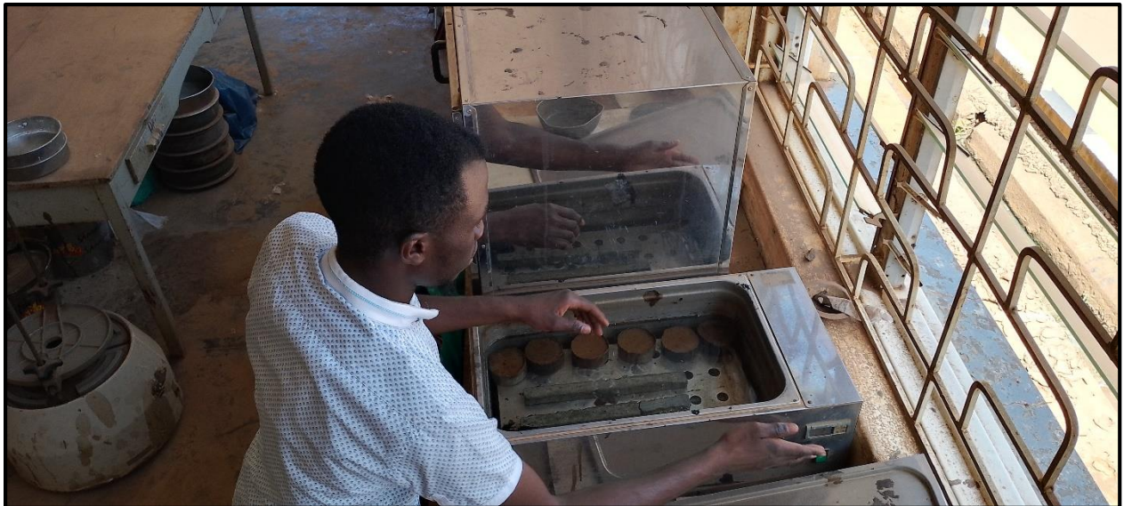
Figure 3-8 Operation of the water bath with concrete prisms/bars for the AMBT.
