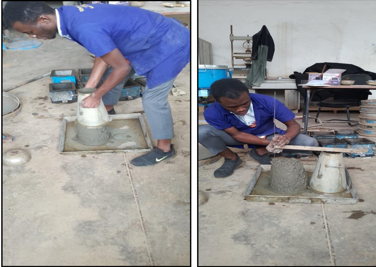
Figure 3-5 Carrying out slump test for freshly mixed concrete.
