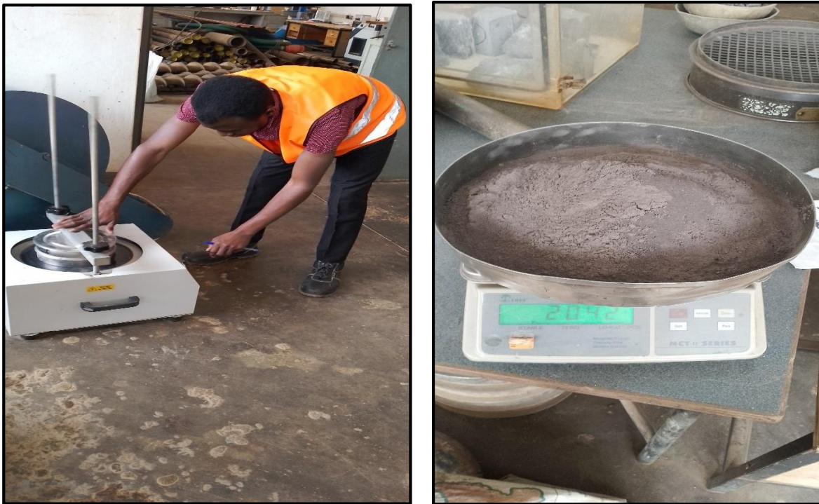
Figure 3-1 Operation of the sieve shaker weighing of pumice powder during sample preparation.
