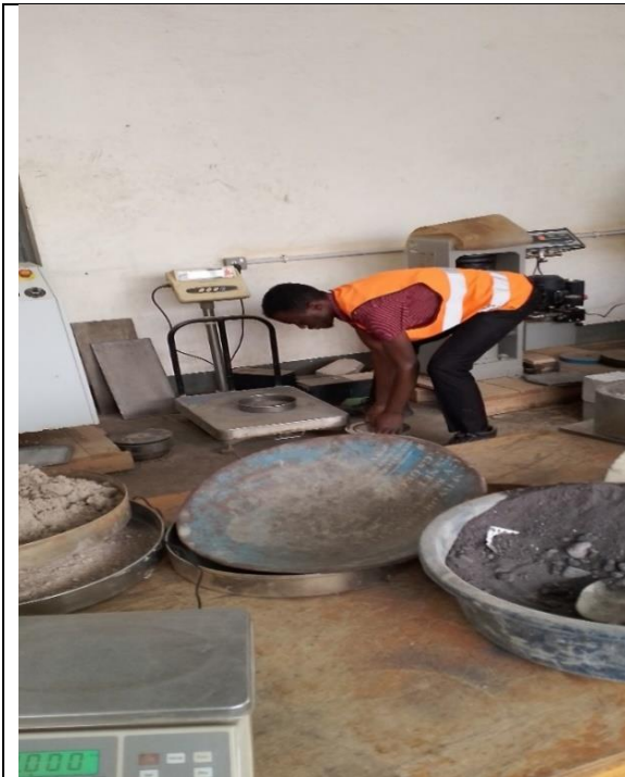
Appendix Figure K-1: Measuring of Pumice powder obtained during sample preparation.
