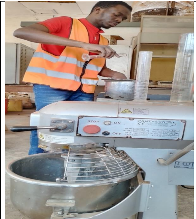
Appendix Figure K-2: Carrying out Consistency & Setting time test for the combination of pumice powder and cement.
