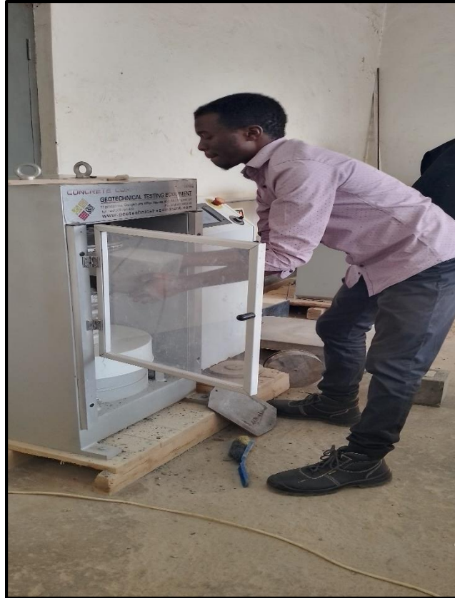
Figure 3-6 Inserting of concrete cubes in the compressive strength machine for crushing.
