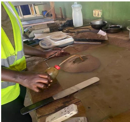
Figure 15. Sample preparation for Atterberg limits test
