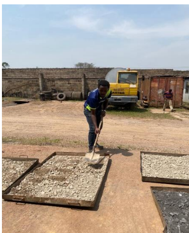
Figure 16. Air drying of granite sample
