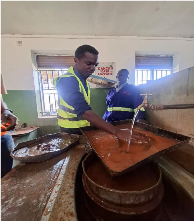
Figure 3: shows washing of soil in preparation for atterberg limits determination
