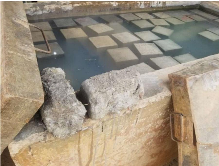
Figure 22 Failed Unfired clay bricks in water absorption test
