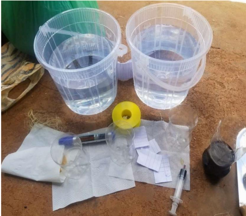
Figure 20 Bio enzyme and proportioning containers
