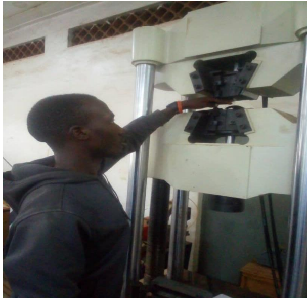
Fixing the PET plastic in the tensile strength testing machine
