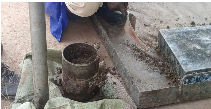
Proctor test during the compaction
