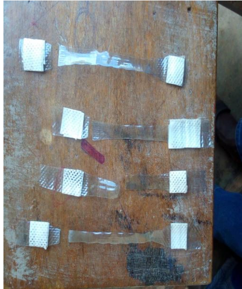
The tested plastics after breaking.
