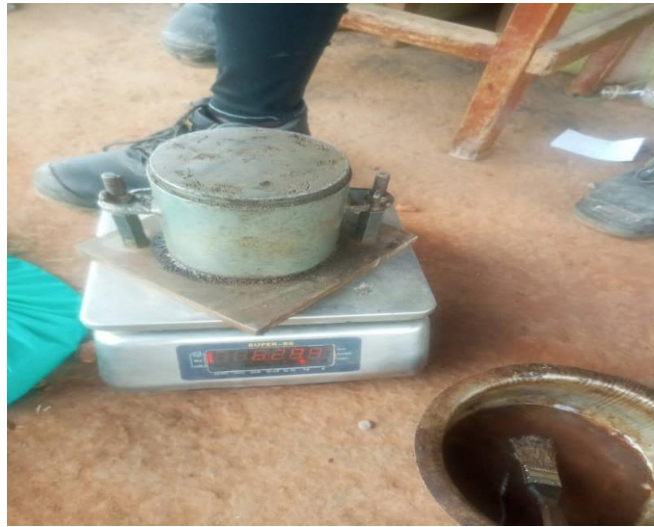
Weighing the compacted soil during the proctor test
