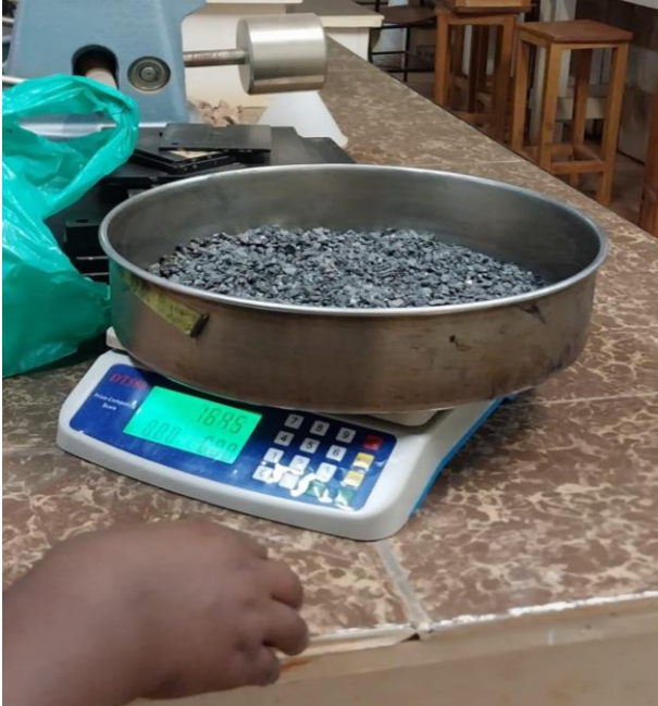
Figure 16: Weighing of steel slag after crushing
