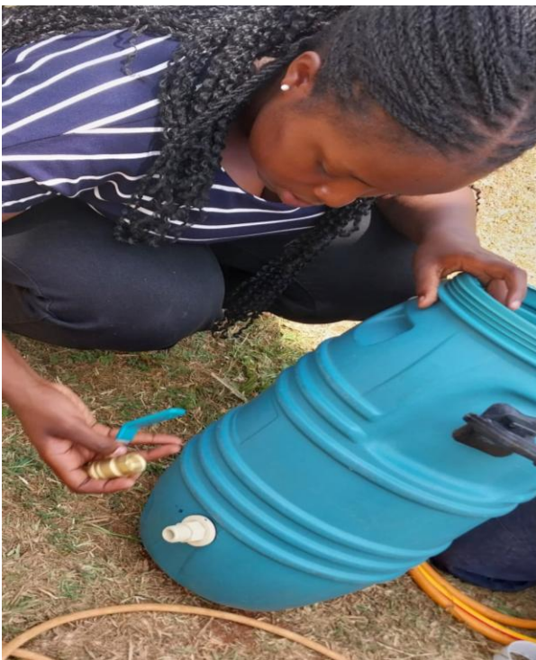
Figure 18: Fabrication of the purification unit
