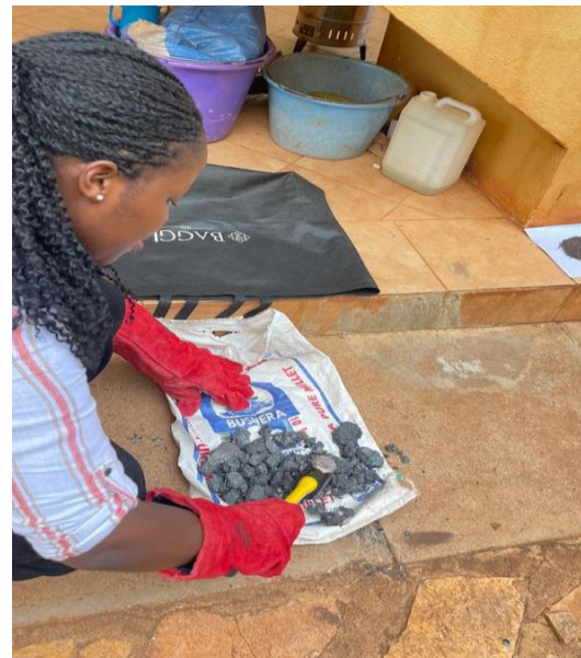
Figure 15: Crushing of steel slag
