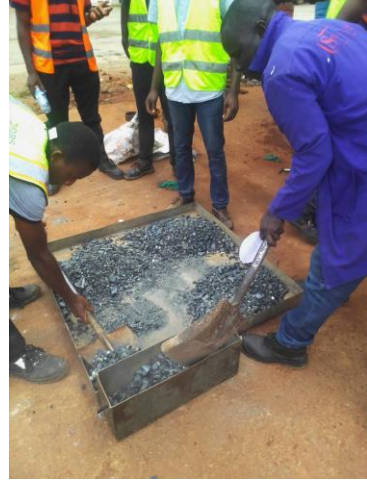
Appendix 2: Quartering of the steel slag
