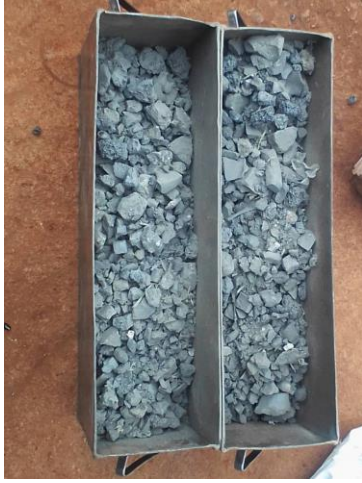
Appendix 1: Riffling of steel slag
