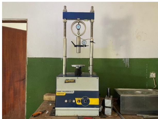
Figure 4: CBR testing machine
