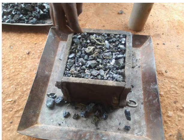
Figure 6: Graduated container filled with steel slag.
