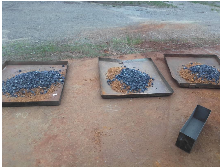
Figure 7: Steel slag added to the neat laterite soil in varying percentages
