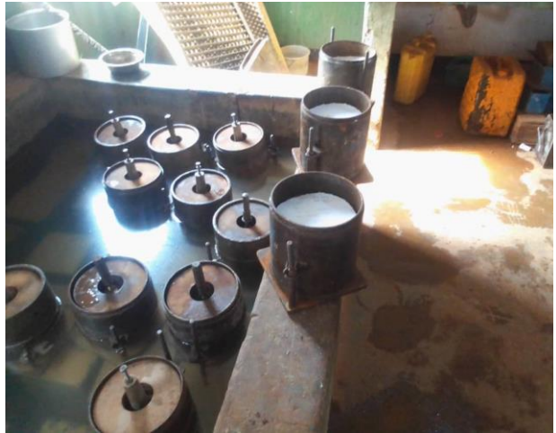
Appendix 6: Soaking tank for CBR swell
