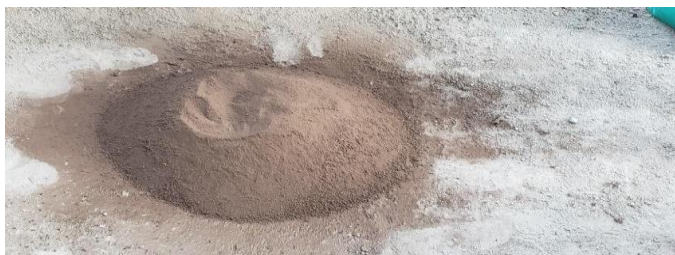
Figure 3: Foundry sand sieved in preparation for concrete mixing
