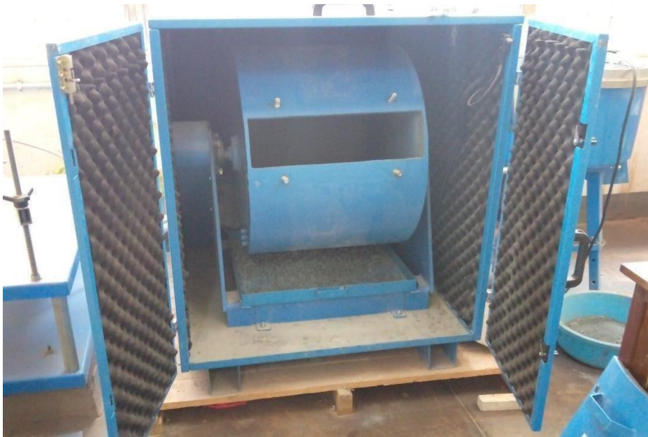
Figure 8: Showing the Los Angeles Abrasion apparatus
