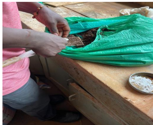
Figure 27: Sample testing for shear box test
