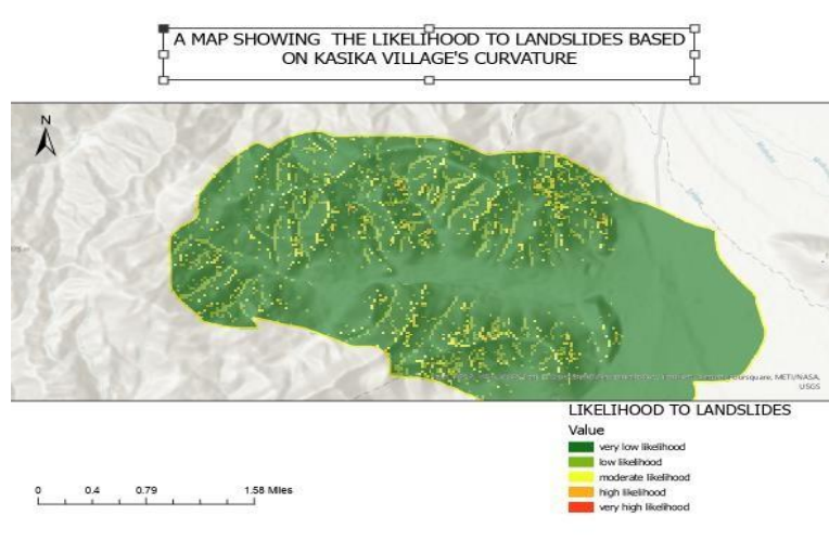
Figure 12: A map showing the reclassified curvature of the slopes in Kasika village
