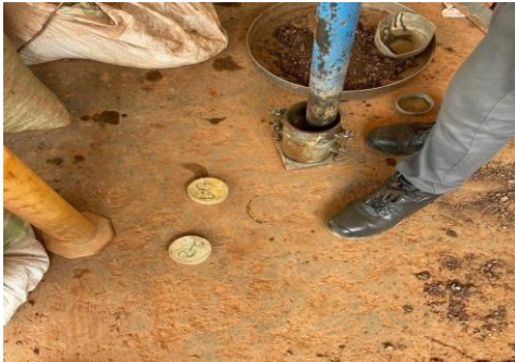
Figure36: Showing compaction in proctor test
