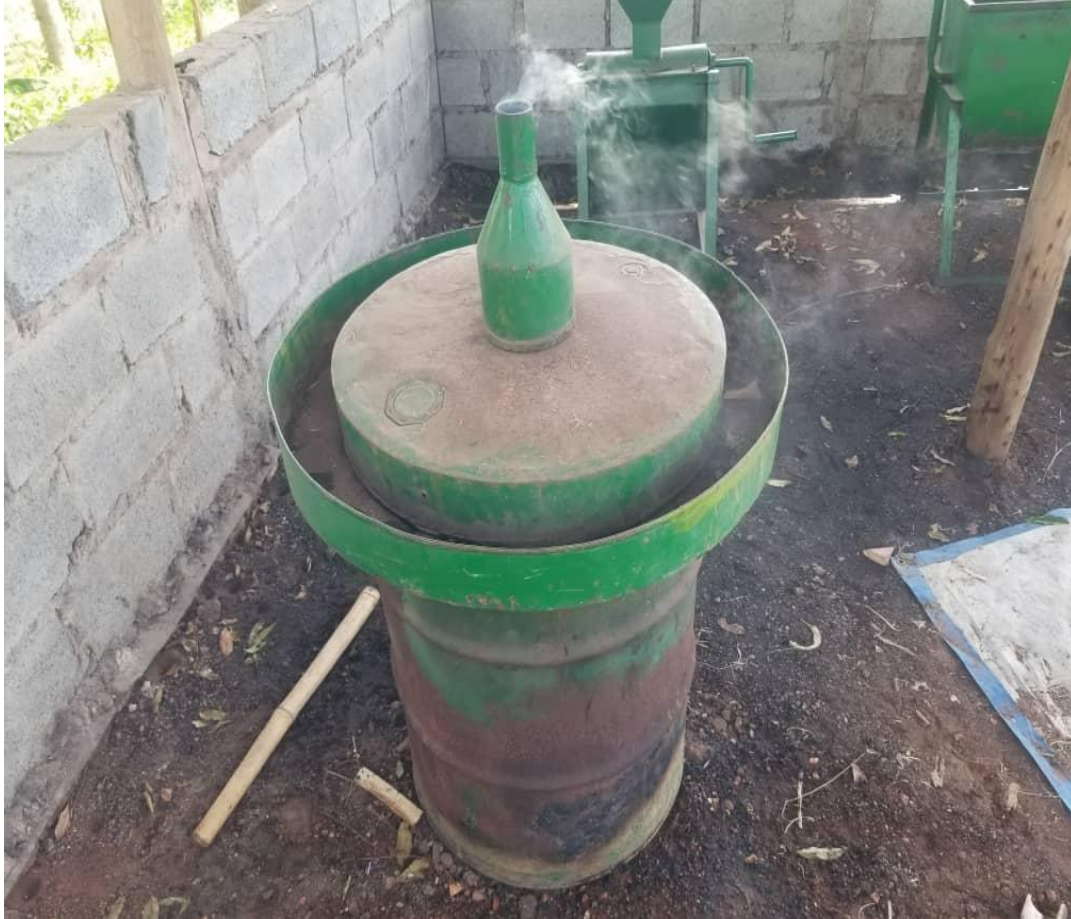
Figure 7: Carbonization of the bamboo
